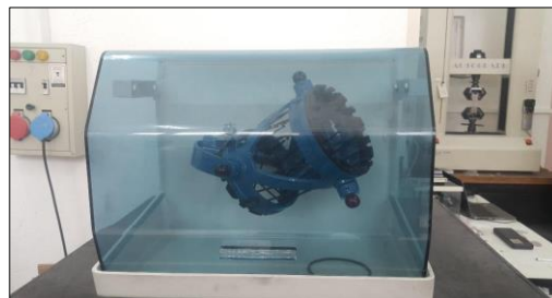
Figure 15. TURBULA T2F device with 3D motion.
