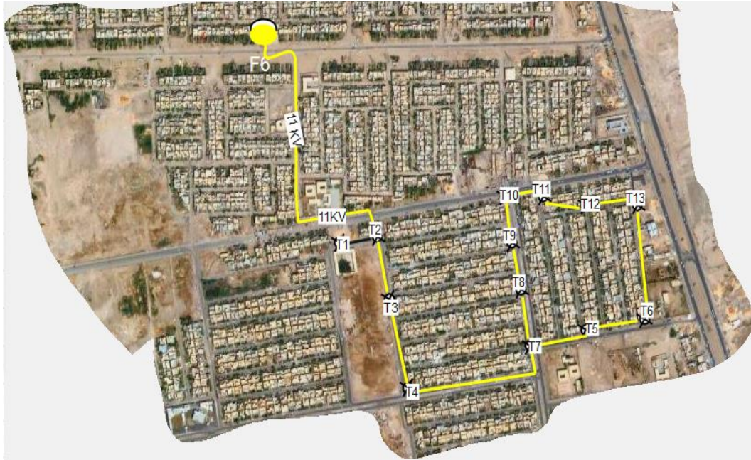
Figure 6.4. Case study of feeder passing (11 kV).
