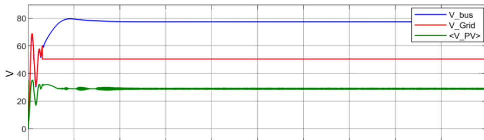
Figure 4.45. System voltage curves in case of 1000 W/m 2 and 25% full load.
