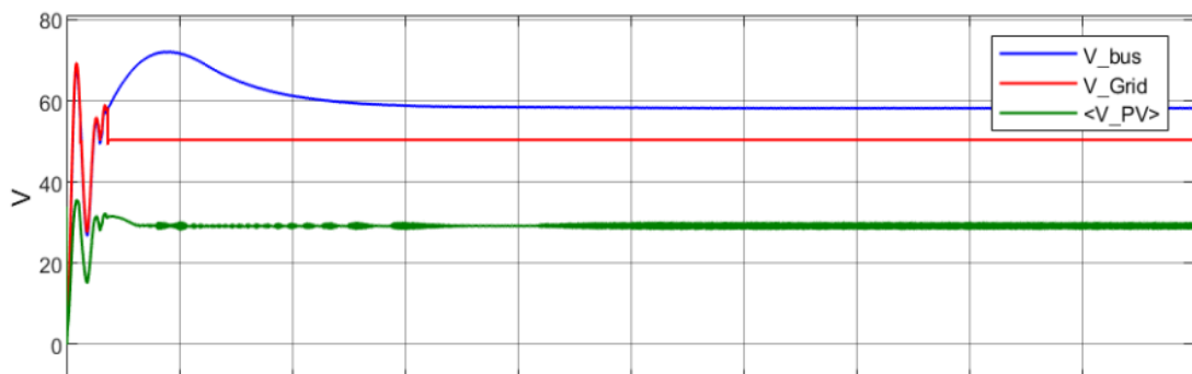
Figure 4.30. System voltage curves in case of 750 W/m 2 and 25% full load.
