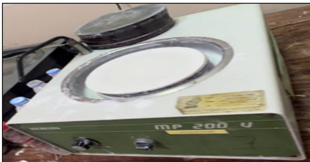
Figure 3.14. The grinding machine.
