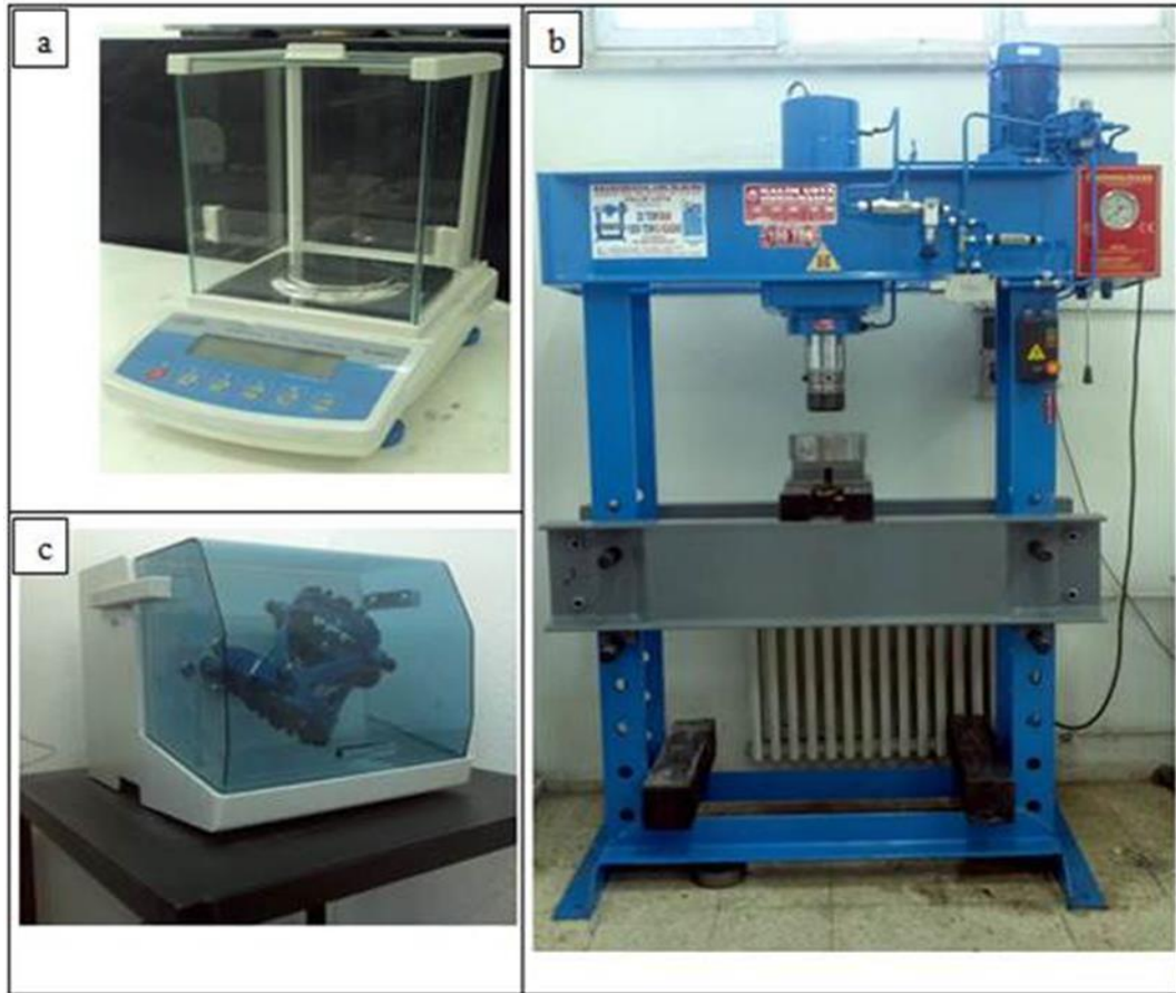
Figure 4.2. Images of a) Precision balance, b) Hydraulic press machine, and c) Powder mixing device used in experimental studies.
