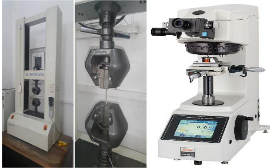
Figure 4.5. SHIMADZU tensile test and hardness measurement device [107].
