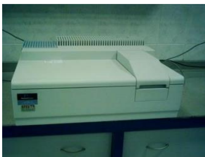
Figure 3.6. The Perkin Elmer Lambda 25 UV-VIS spectrometer.
