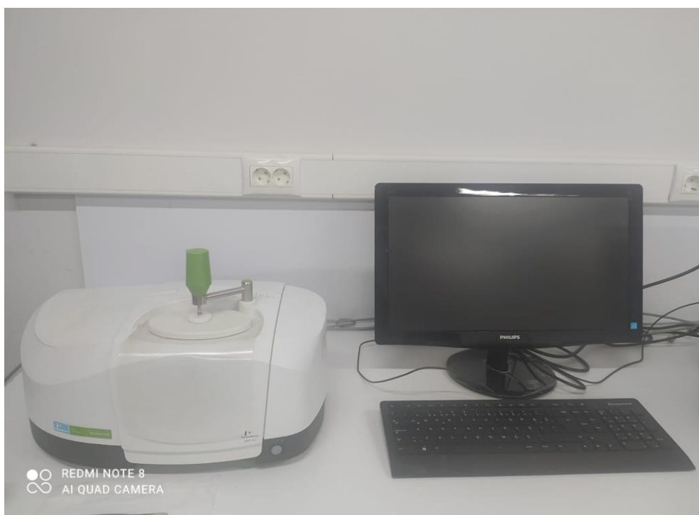
Figure 3.7. Parkin Elmer spectra FT-IR Spectrophotometer at Usak University [30].
