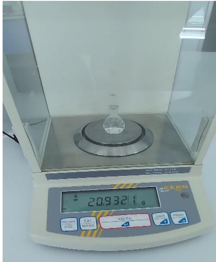
Figure 3.3. Density measurement using Pycnometric method at Chemical Engineering Laboratory, Faculty of Engineering, Usak University.
