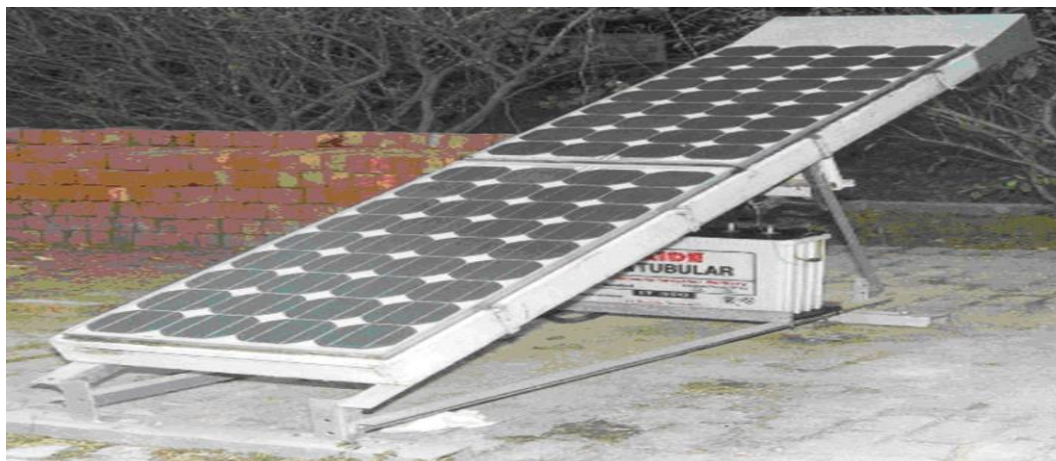
Figure 2.2. Hybrid solar collector with single pass (PV/T) [8].
