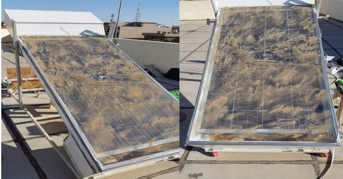
Figure 2.4. Collector (PV/T) in case of dust [18].
