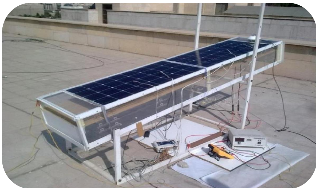
Figure 2.6. Hybrid solar collector (PV/T) [21].
