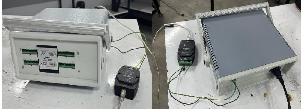
Figure 4.18. Ordel brand UDL200-05/20 data logger [119].
