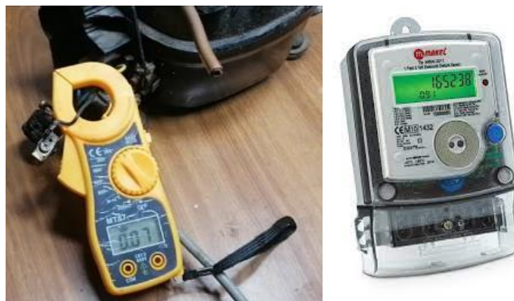
Figure 4.19. Makel M310.2218, single phase, electronic electricity meter, Current measurement application with a clamp meter.
