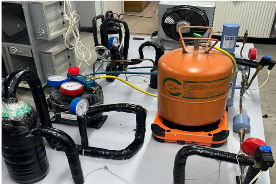
Figure 4.15. Vacuum test and gas charge to the MCRS.
