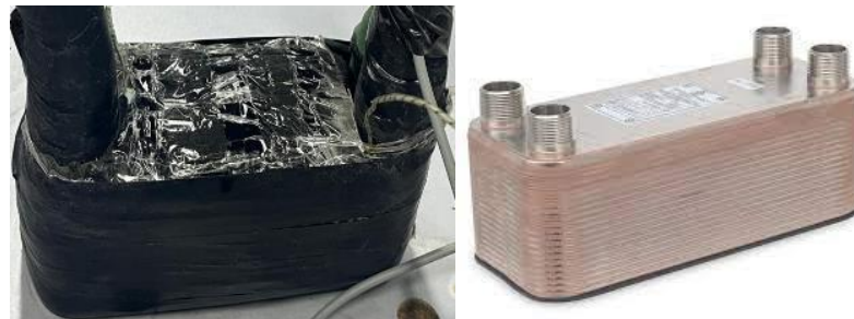
Figure 4.10. HEX Before and After thermal insulation.
