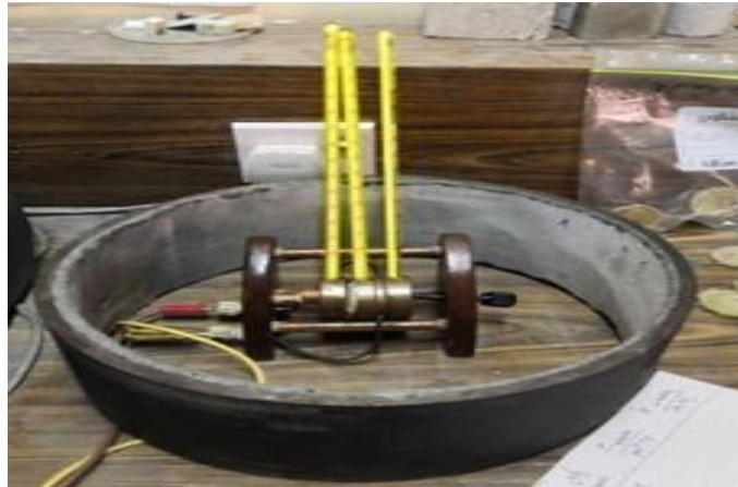
Figure 3.7. Lee's disc method.
