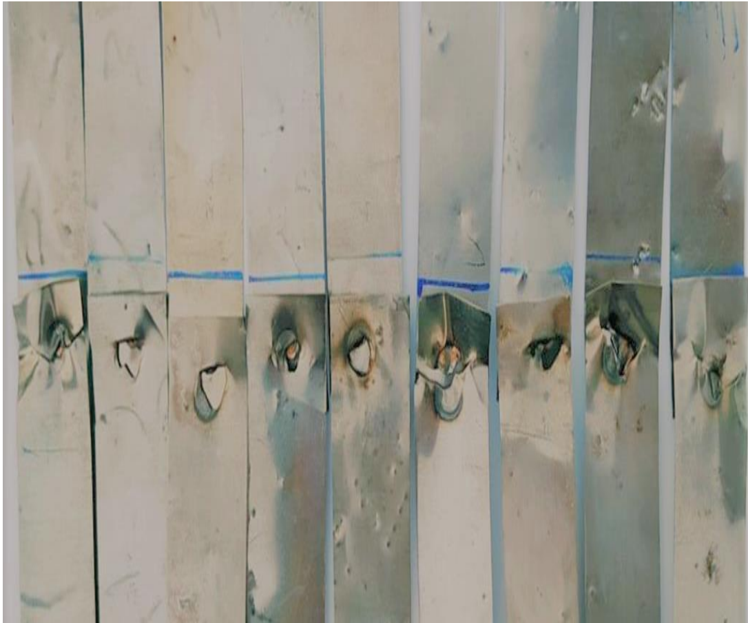
Figure 5.2. Failure specimens after shear test.
