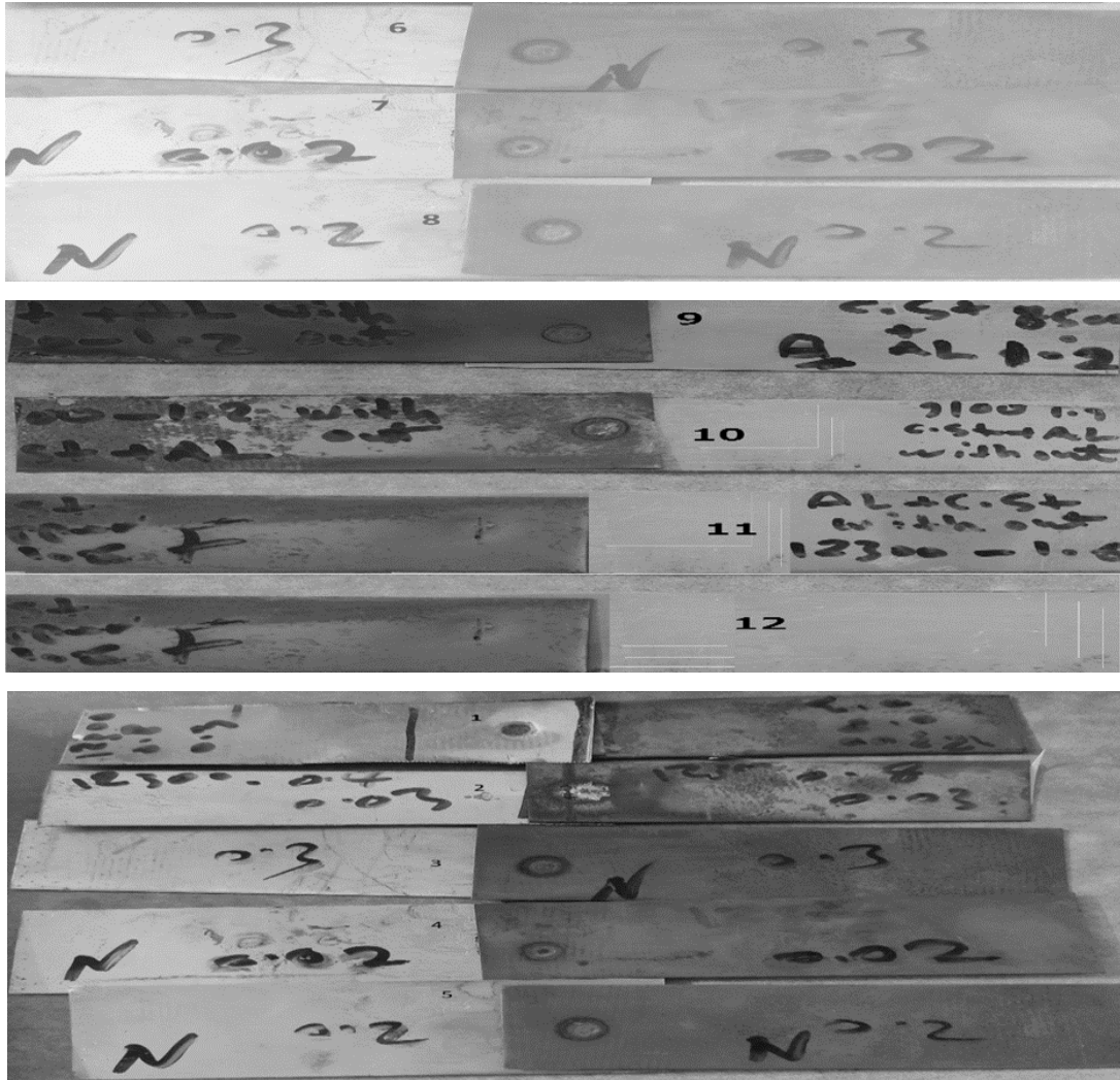
Figure 5.3. Specimens before shear test of metal interlayer.
