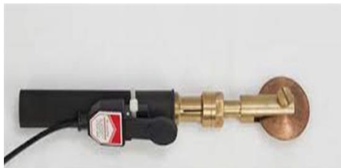
Figure 3.7. Roll spot welding process.
