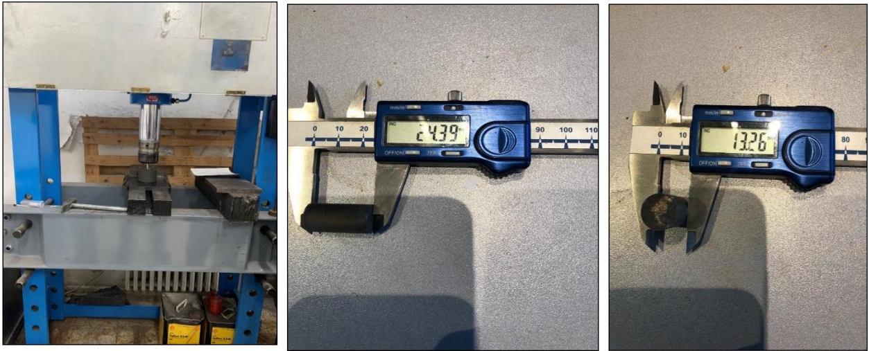
Figure 4.3. The sample's pressing, mold, and diameter.
