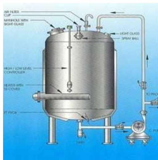
Figure 3.9. Schematic of storage tank type fully mixed [28].
