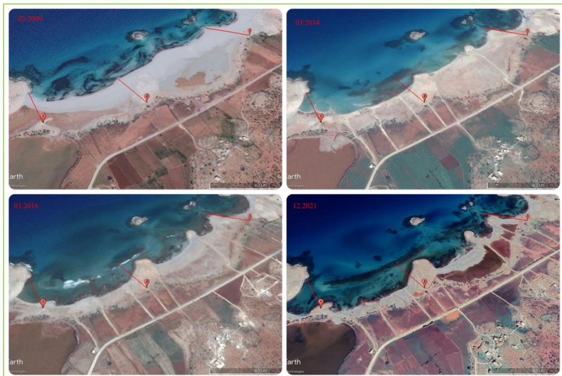
Picture 105. Coastal dune erosion due to extreme sand dredging between 2009 and 2021
