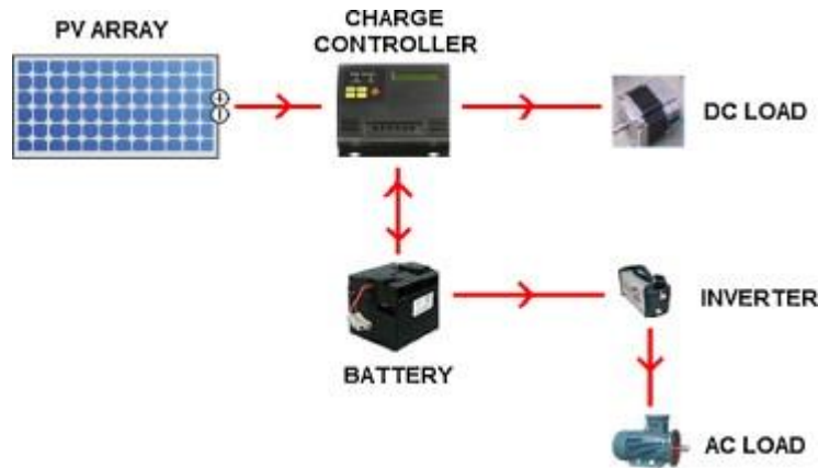
Figure 1. 14. Diagram of the simplified off-grid PV system [28].
