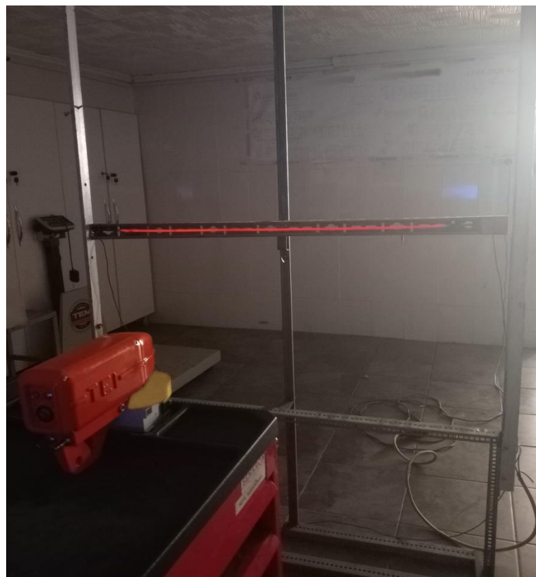
Figure 5.15. Loop scanner detecting resistance wire.
