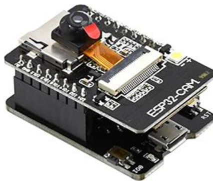
Figure 5.5. ESP32 cam module.
