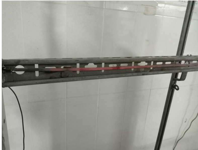
Figure 5.14. Resistance wire used in mechanical setup.
