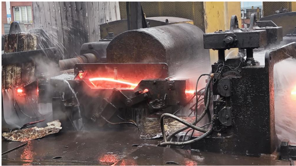
Figure 3.8. Loop formation in hot rolling mill.
