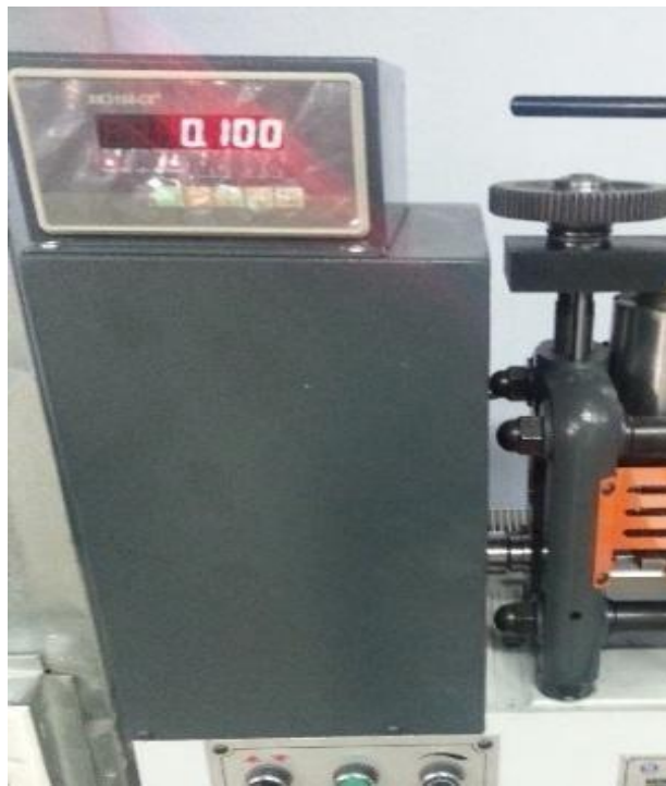
Figure 4.5. Screen displaying the rolling force measured by the load cell.
