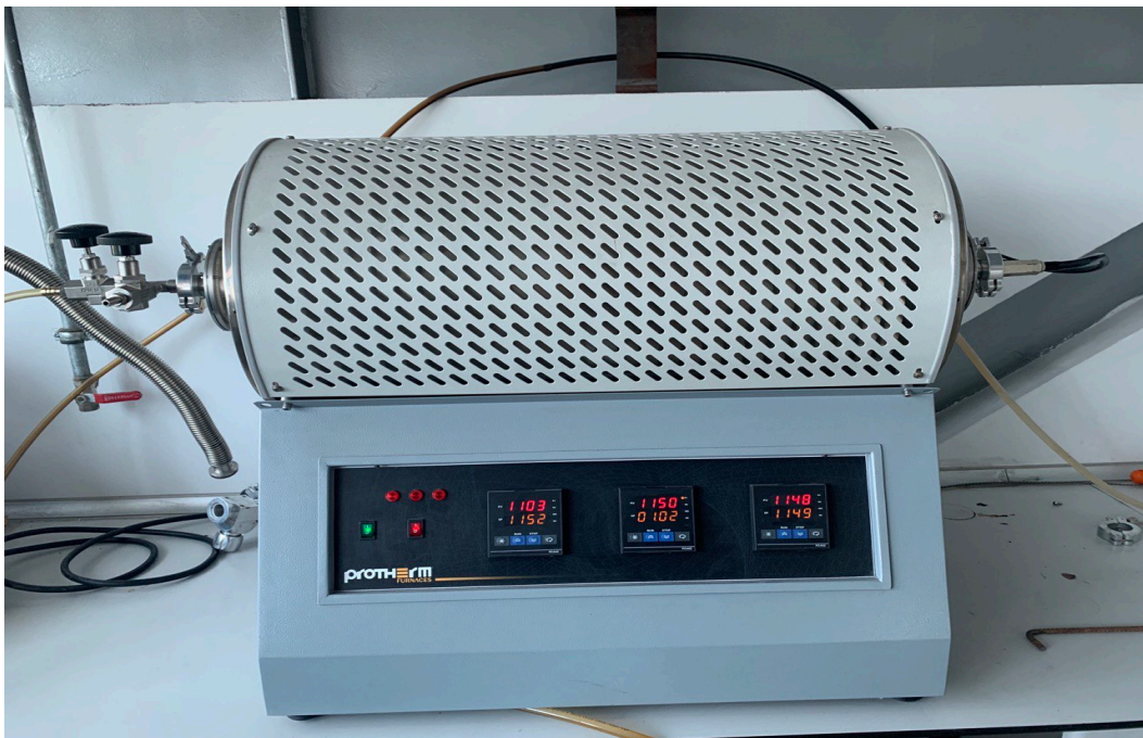
Figure 4.6 Atmosphere-controlled Tube Furnace used for the sintering process.
