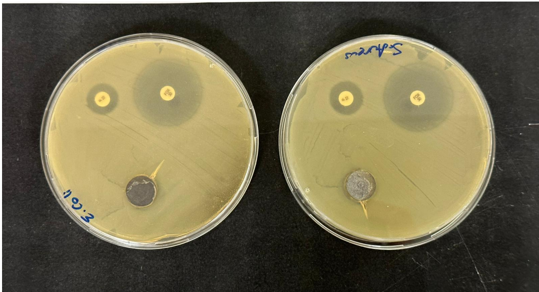
Figure 5.14. Inhibition zone of the S.Aureus (25923) and E.Coli (25922) inoculated bacteria plate with the Ti-15Mo-2In sample.
