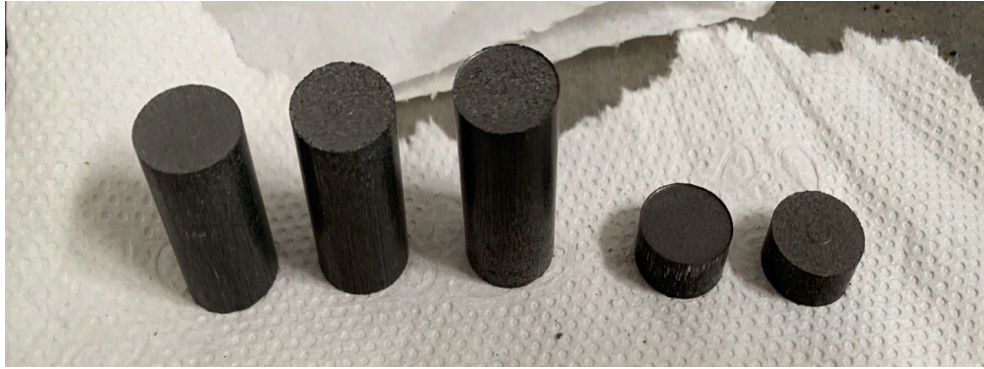
Figure 4.5. Different sizes of specimens (13 mm x 26 mm and 13 mm x 5 mm).
