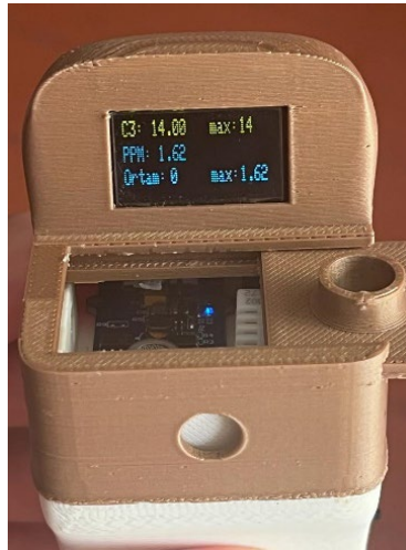
Figure 4.6. The BBGM device measuring BA value in ppm.
