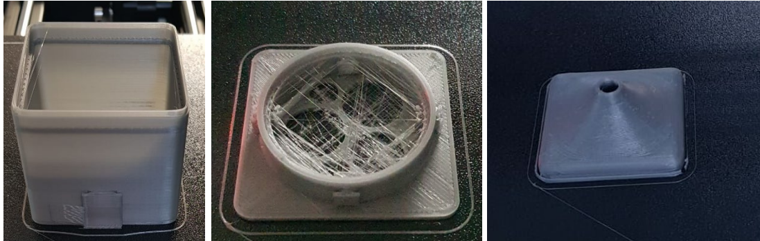
Figure 3.9. The test device parts printed with a 3D printer.
