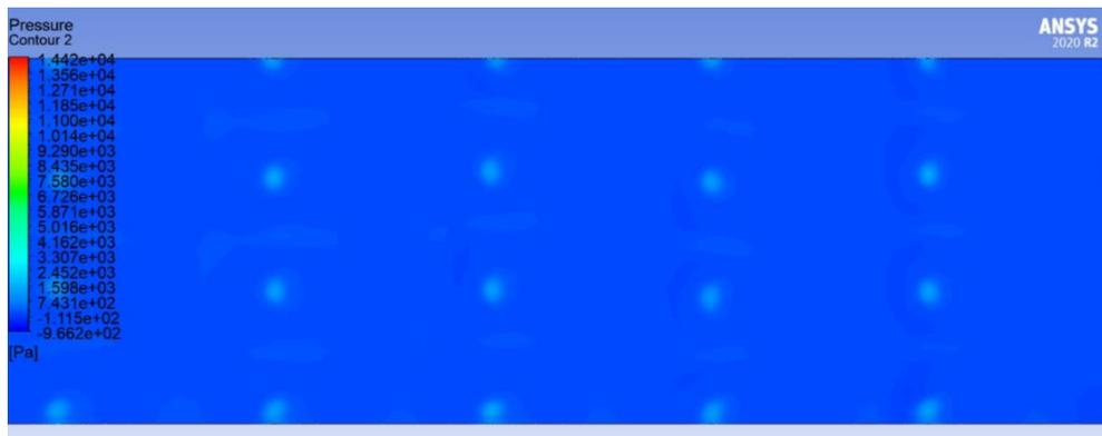
Figure 3.22. Top view of pressure distribution on the smooth absorber.
