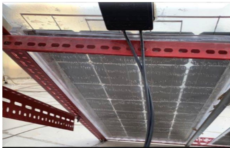
Figure 4.7. The porous media plate inserted in the perspex container backside of the cooled photovoltaic panel.
