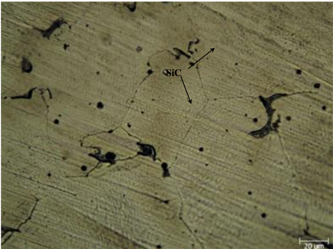
(g) ZK60II at 500 X after casting.
