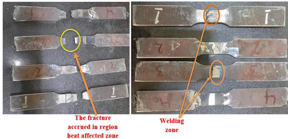
Figure 5.9. Tensile specimens, before and after the tensile test.
