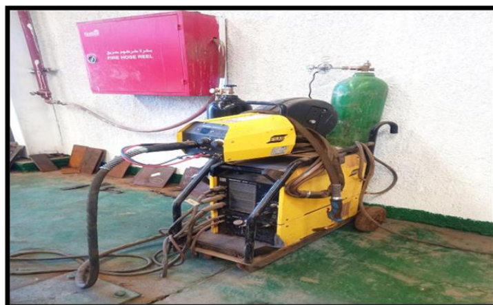
Figure 4.4. The MIG welder used for this task.
