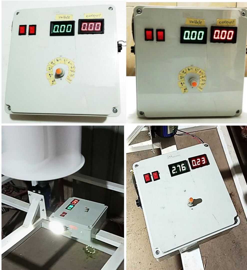
Figure 3.15. Current and voltage measuring device.
