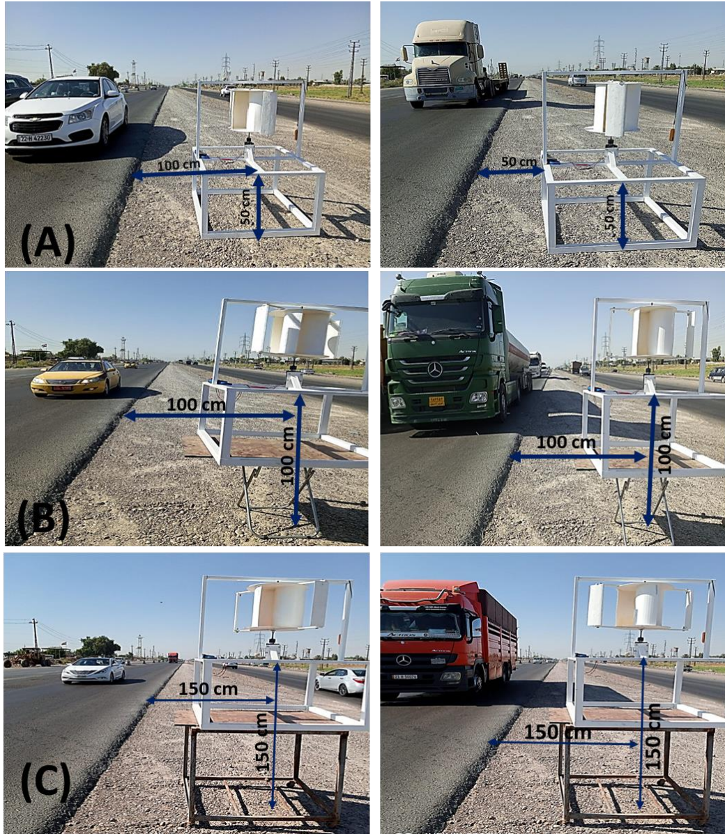
Figure 3.25. Height tests for a double turbine at (A): Test G, (B): Test H, (C): Test I.
