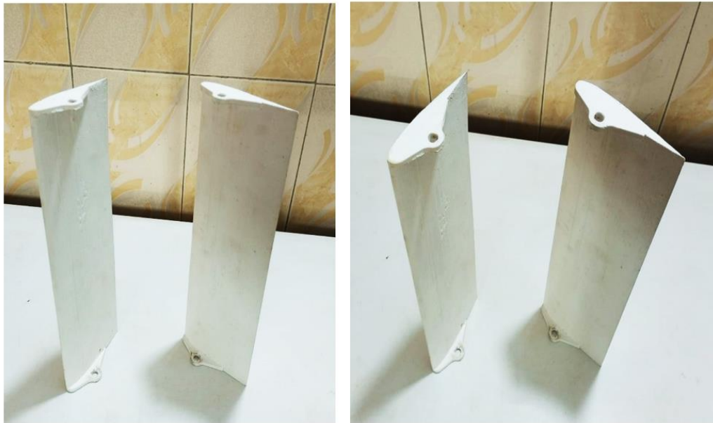
Figure 3.6. Manufacturing of Darrius Blades.
