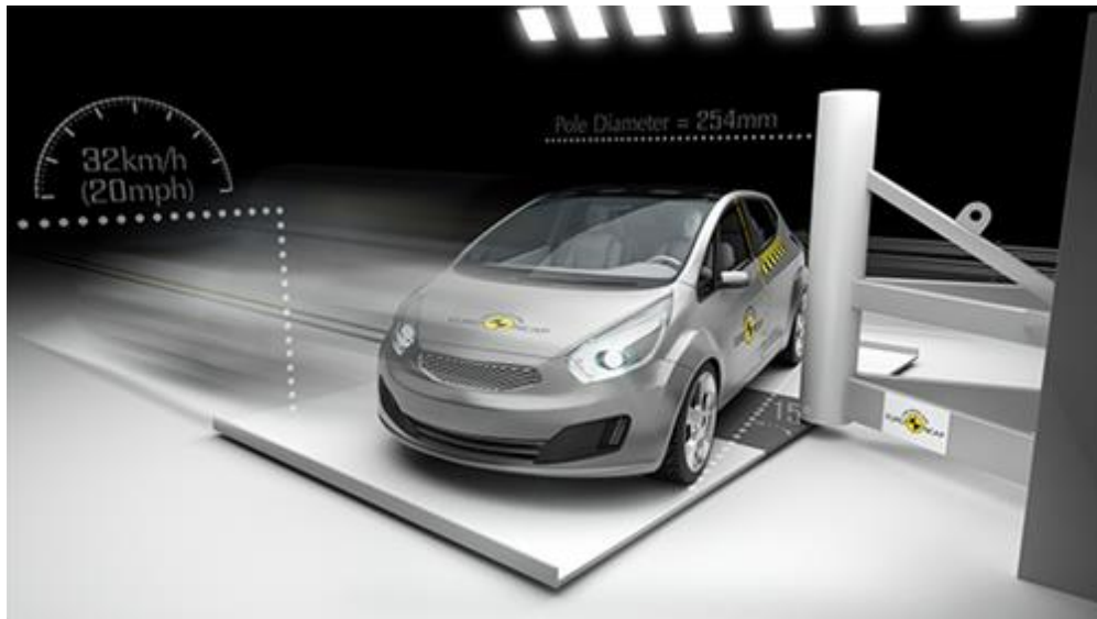
Figure 1.12. Lateral collision test between test car and rigid pole.
