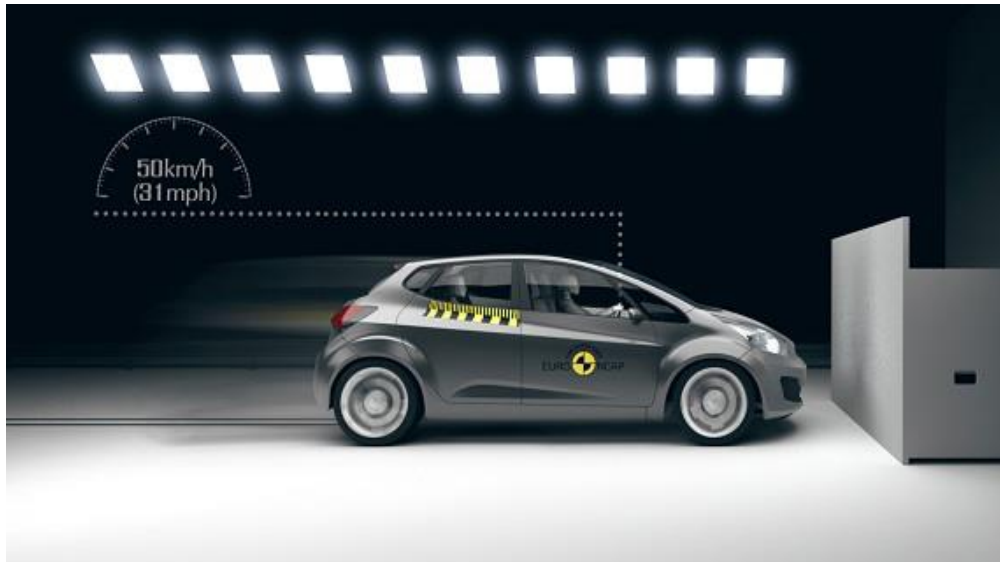
Figure 1.9. Full width collision of a vehicle tested by Euro NCAP with a rigid wall.
