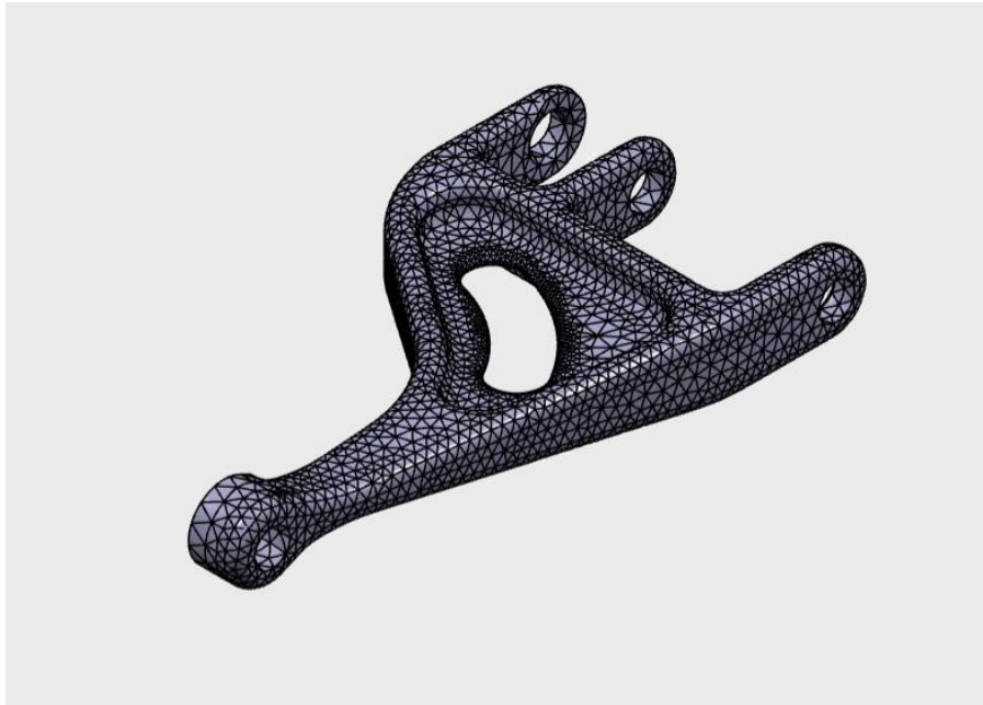
Figure 3.3. FEM appearance of the mechanical part to be simulated in the pre-processing stage.
