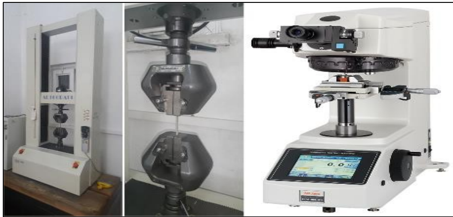
Figure 5.5. SHIMADZU tensile test and hardness measurement device [107].
