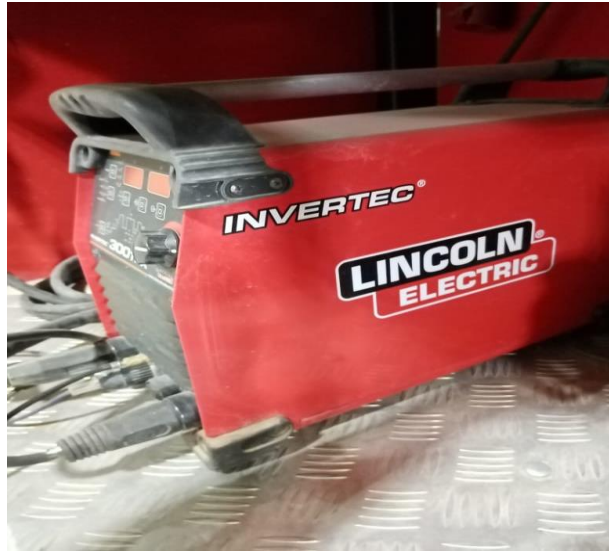
Figure 4.2. Welding machine (TIG).
