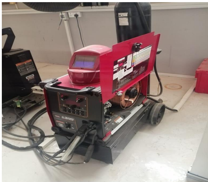
Figure 4.1. Welding machine (MIG/MAG).
