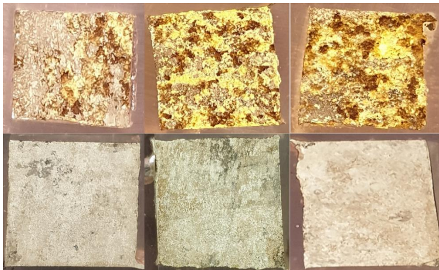
Figure 4.19. Image of the prepared samples after polarization analysis in HBSS + solution.
