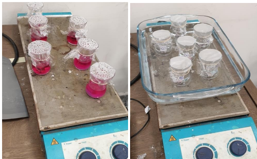
Figure 3.9. Immersion test of AZ31 alloys.
