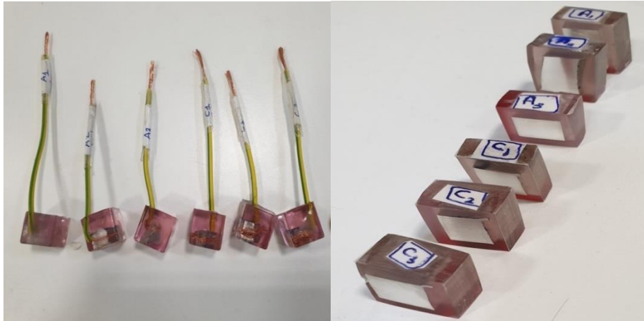
Figure 3.5. The cold bakelite mold for the prepared samples.
