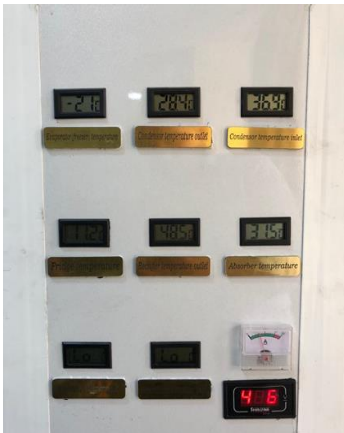
Thermal sensor panel linked to the various components of the refrigerator.
