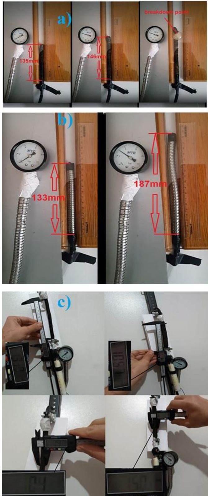
Figure 4.1. Muscle with different covers: a) nylon spiral, b) metallic spiral, and c) polyester mesh cover.
