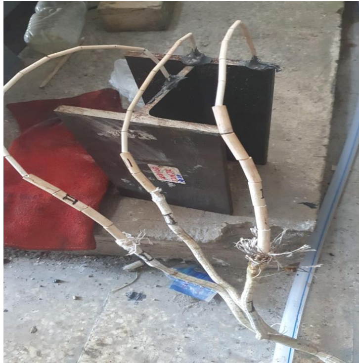
Figure 3.3. Thermocouple mounted profile.
