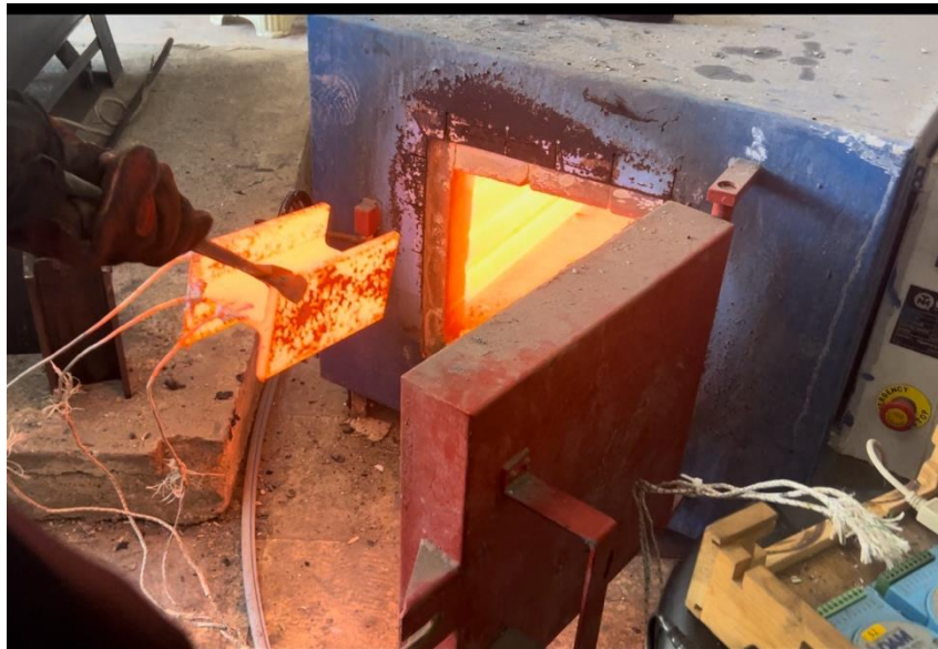
Figure 3.5. Heat treatment furnace .
