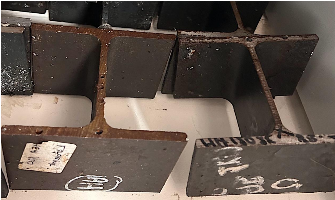
Figure 3.2. Positions of holes drilled for thermocouples.
