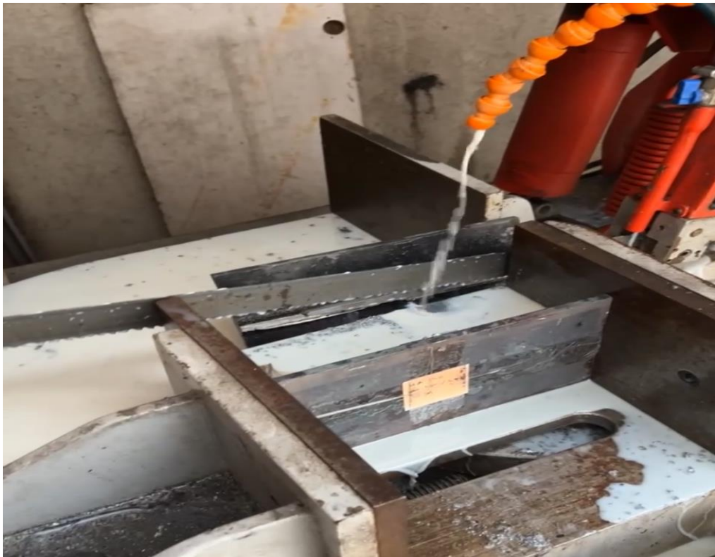
Figure 3.1. Cutting profiles to a length of 250 mm.
