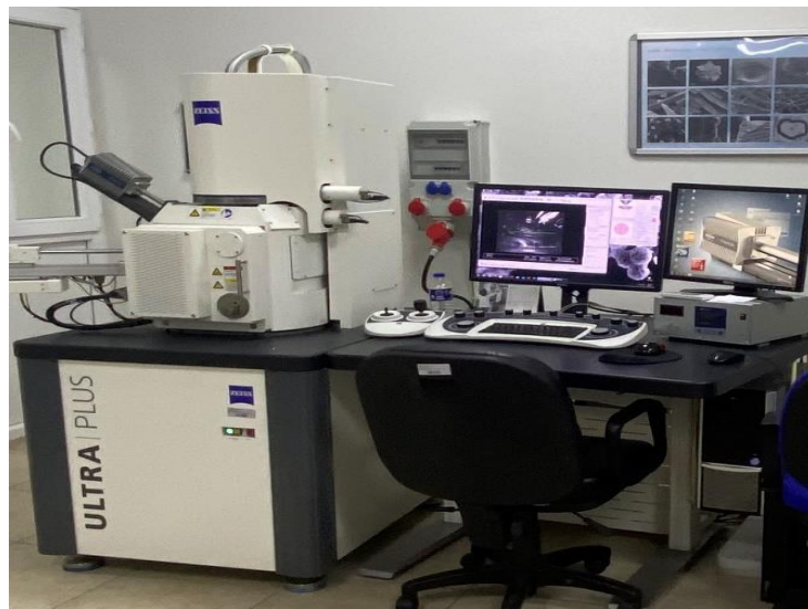
Figure 4.10. (SEM) The scanning electron microscope, and (EDS) energy dispersed element analysis.
