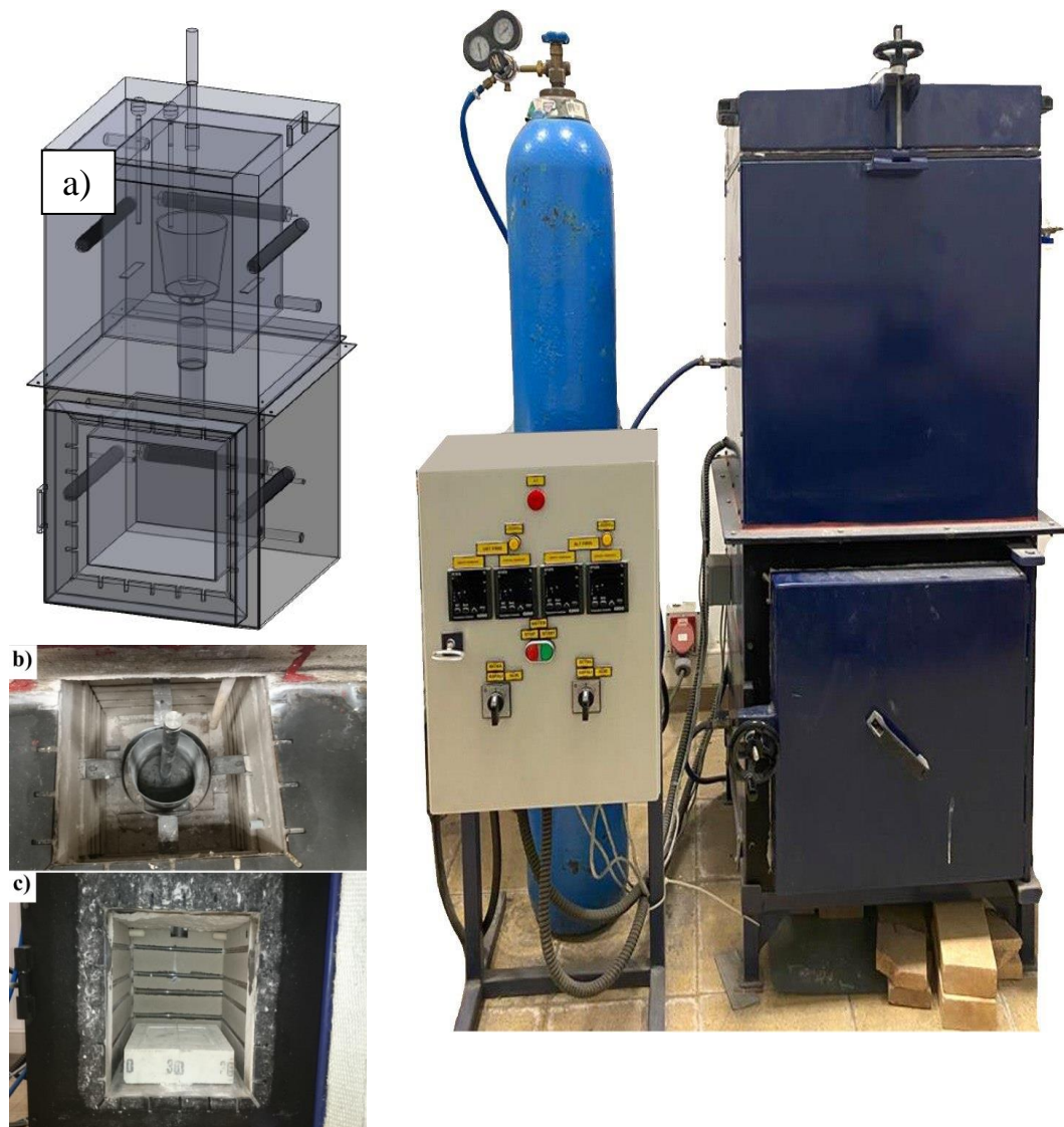
Figure 4.1. The casting furnaces.
