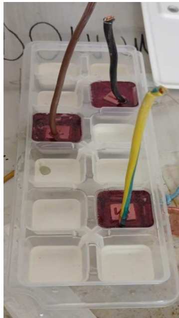
Figure 4 2. Sample after the cold bakelite process
