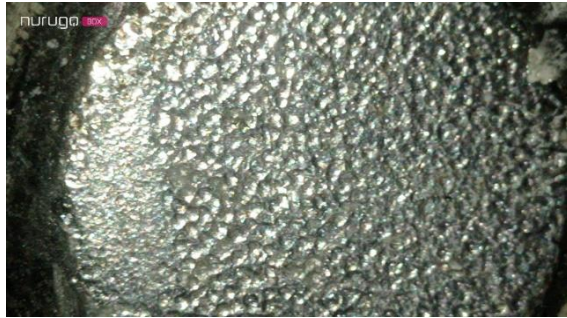
Figure 4 3. Sample surface after Shoot peening process
