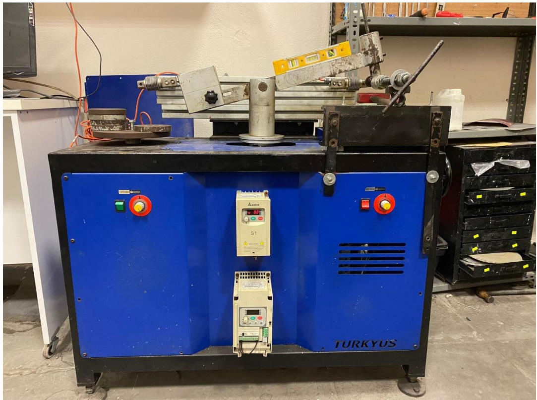
Figure 3.5. AISI 52100 steel ball abrasion tester.
