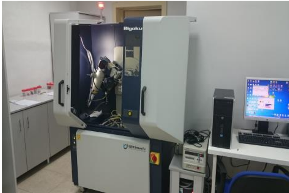
Figure 3.2. X-Ray Diffraction Spectrometer measuring instrument: Rigaku Ultima IV.
