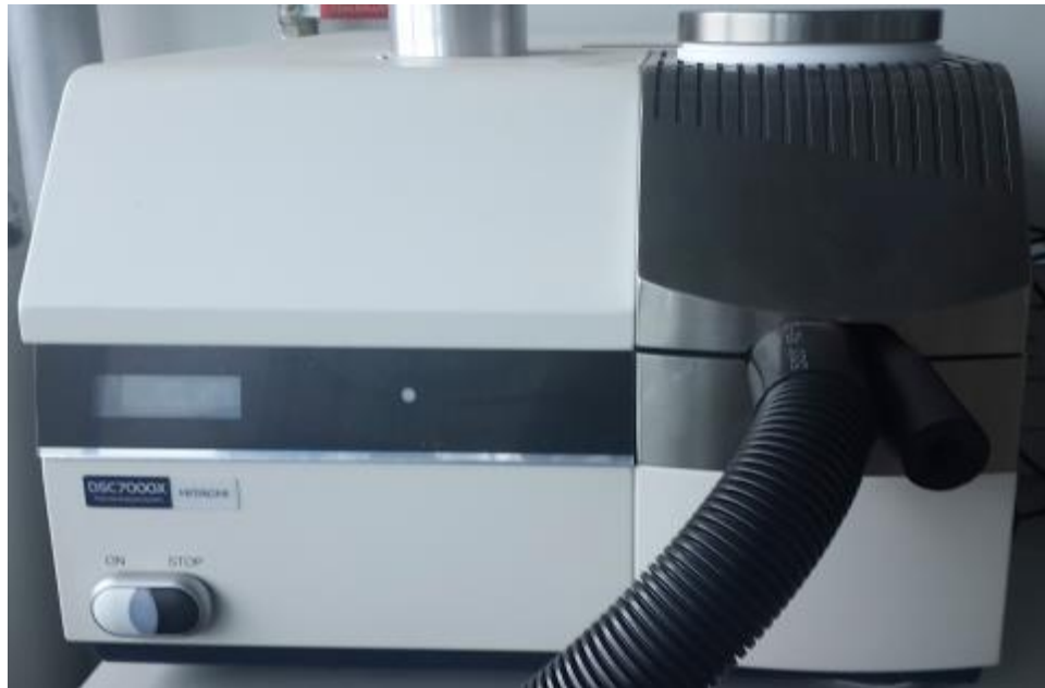
Figure 3.6. Hitachi Differential Scanning Calorimeter.
