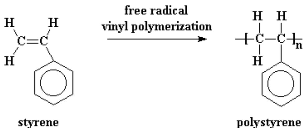
Figure 3.2. Formation of polystyrene by the polymerization reaction of styrene monomer [26].
