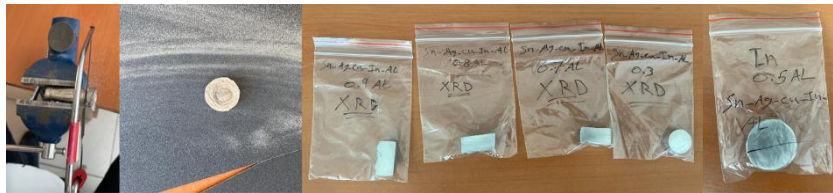
Figure 4.4. Preparing the samples for XRF and XRD analysis.
