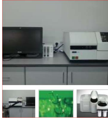
Figure 4.6. DTA/TGA/DSC Laboratory for determining melting temperature of solder alloys.
