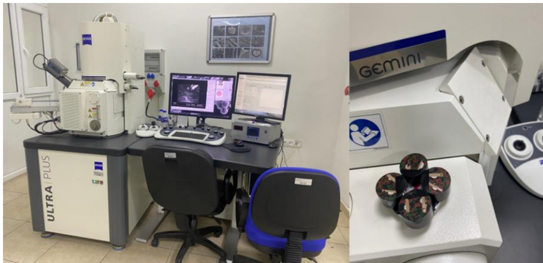
Figure 4.8. The device used for the SEM-EDX analysis " ZEISS ULTRA PLUS FESEM SE2.
