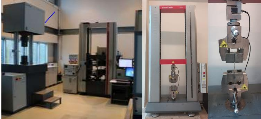
Figure 4.13. The device used for shear strength test Zwick Roell Z050 device at static test laboratory of Karabük University Iron and Steel Institute.
