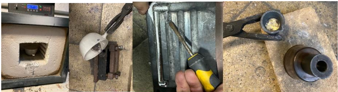
Figure 4.1. Melting materials in a controlled atmosphere unit (Furnace).
