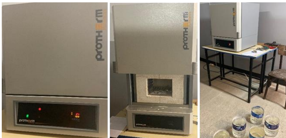
Figure 4.3. Electric furnace used for homogenization process
