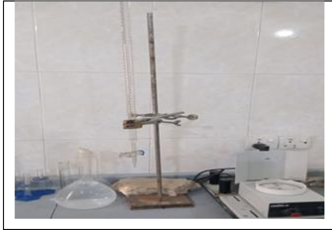
Figure 5. 4. Burette device to measure cations and anions
