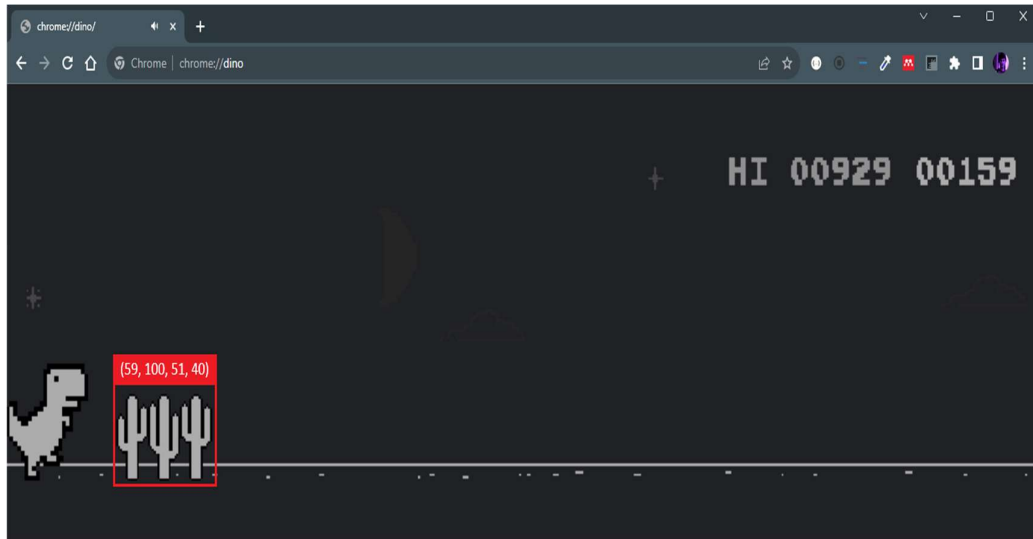
Figure 5.5. A snapshot of the Chrome Dino Run game environment, that shows how it give the precise coordinates and also the dimensions of the obstacle in the game.
