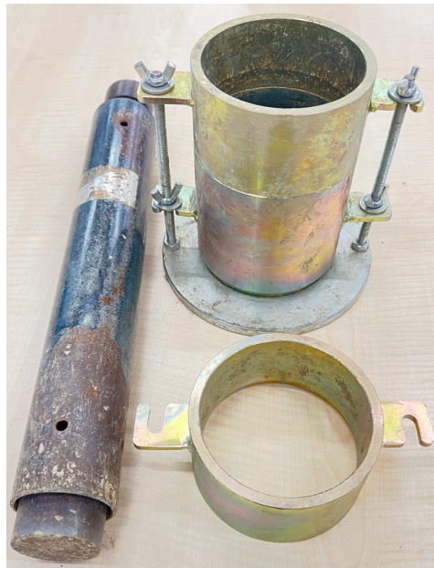
Figure 0.7. The manual compaction device
