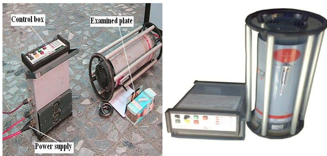
Figure 4.14. X-Ray examination system.
