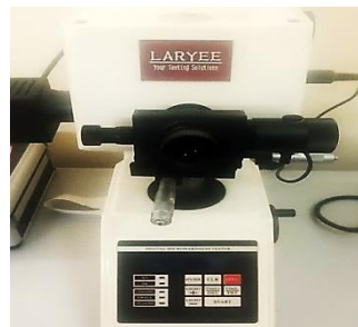
Figure 4.23. Micro hardness test apparatus and microhardness specimens
