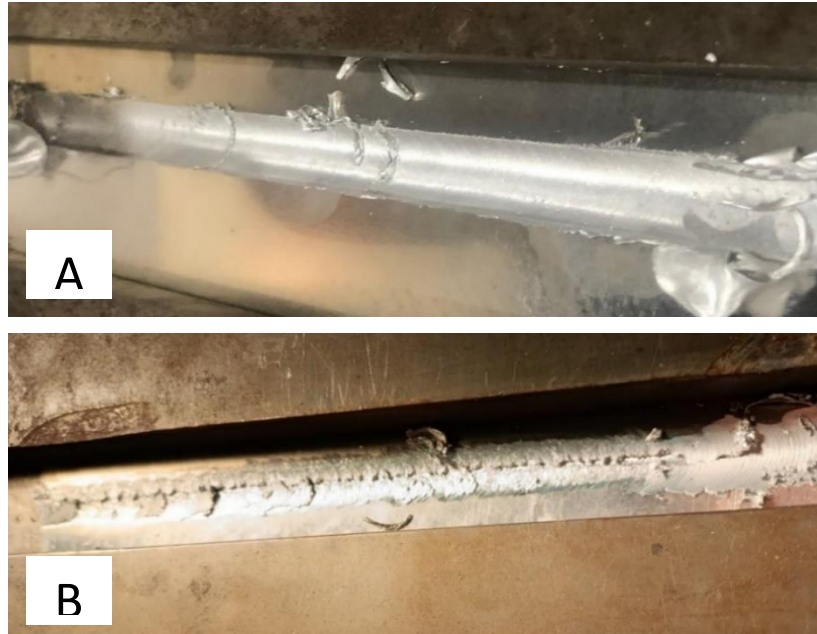
Figure 5. 1. Surface visual inspection of weldments; (a) similar weld AA6061-T6 at 1400 RPM and 45mm/min (b) dissimilar weld at 450 RPM with 71mm/min.
