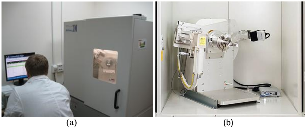
Figure 4.15. (a) XRD device, and (b) X-ray diffractometer
