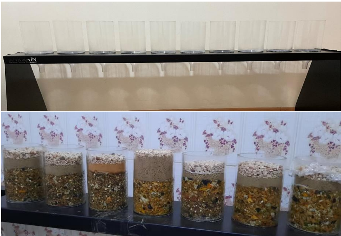
Figure 3.26. The actual setup of the column models before and after being filled with the materials
