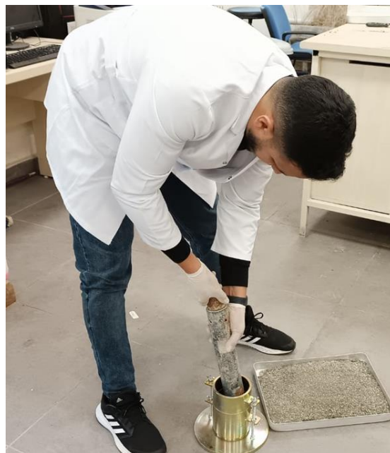
Figure 3.11. Applying the standard compaction test on the clayey samples
