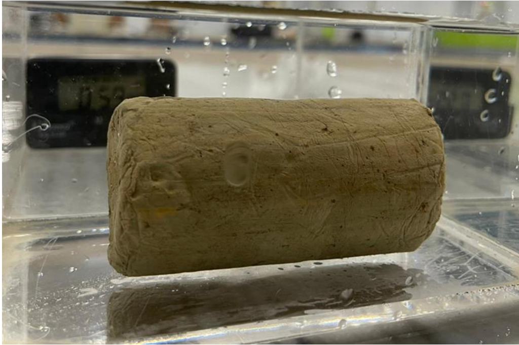
Figure 3.12. Compacted clay sample submerged in water
