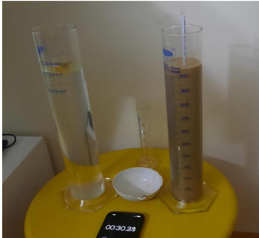
Figure 3.4. A view of the hydrometer test performed on the clayey sample in the lab
