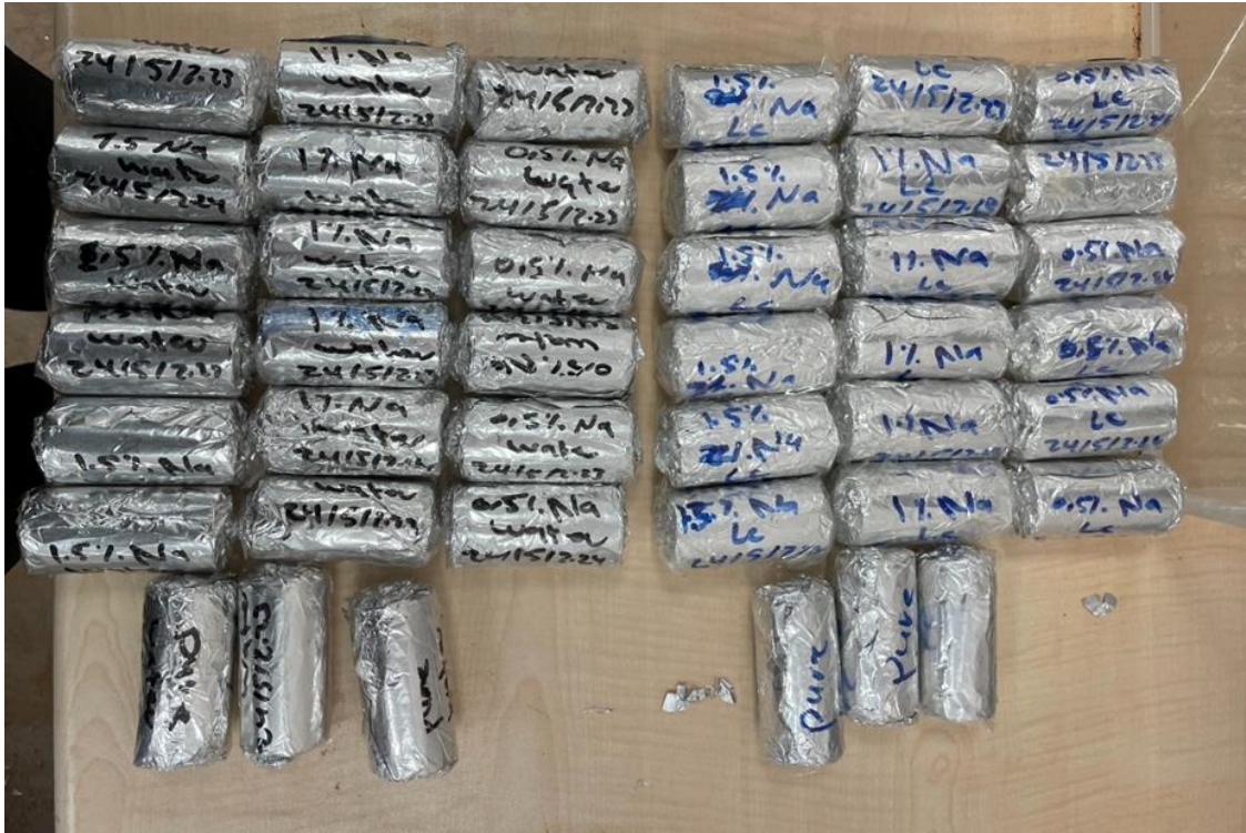
Figure 3.16. UCS and BE samples provided for the study
