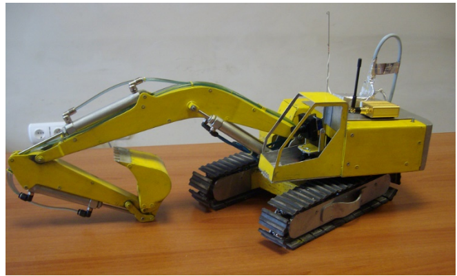
Figure 4: Manufactured excavator robot.
