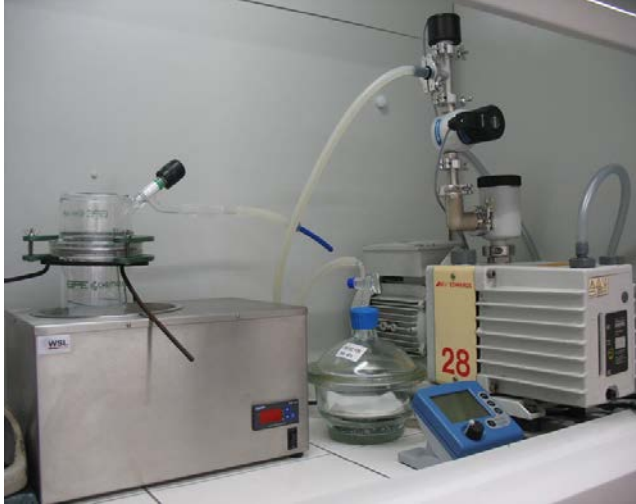
Figure 8: Tissue coating with sublimation method.
