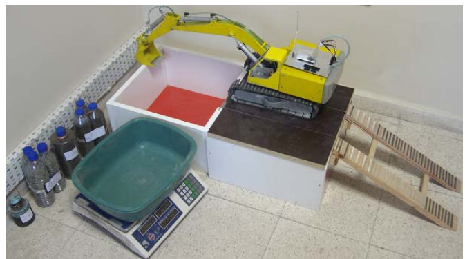
Figure 8: Experimental environment In canal excavation application, the operator takes the soil
