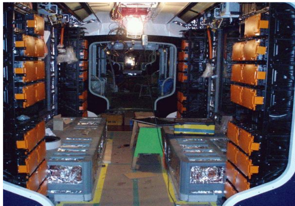
Figure 12. Li-Polymer battery in the Tram [16]
