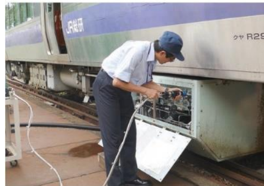
Figure 6. Filling up the hydrogen storage tank with hydrogen [5].
