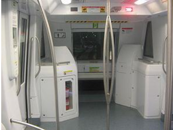
Figure 16. Figure 1. An automated metro system without train driver (Barcelona Metro line 9) [23]
