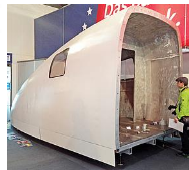
Figure 8. High speed train cab assembled from aluminium foam
