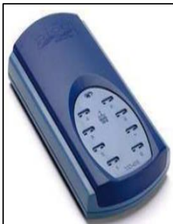
Figure 4.5. Data Collection System (Pico thermocouple data logger TC-08).
