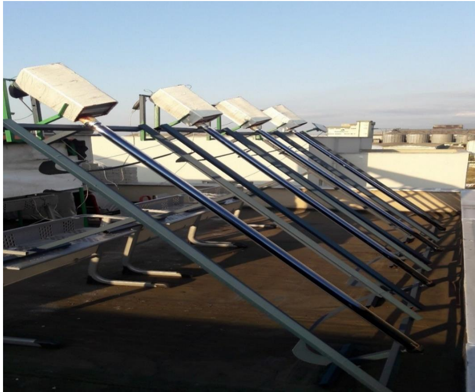
Figure 3.8. Photograph showing the heat pipes receives solar radiation at an angle of 41°.
