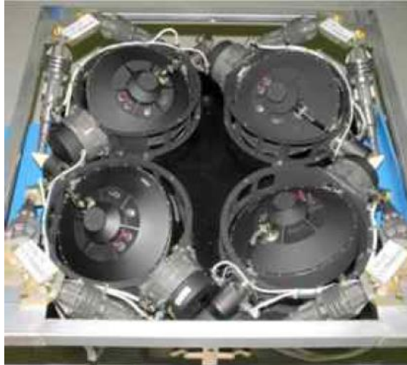
Figure 2.4b. Operational principle CMG [20].
