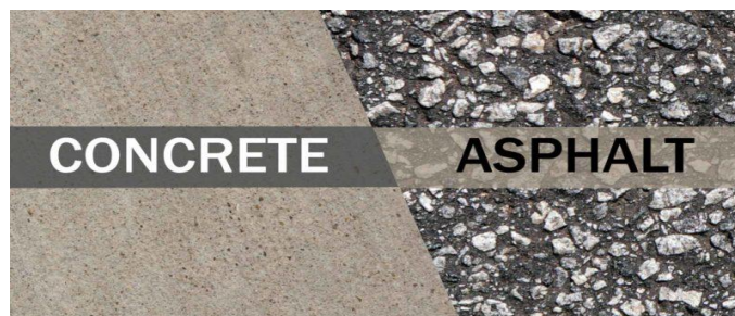
Figure 3.1. Flexible pavement and rigid pavement [47].
