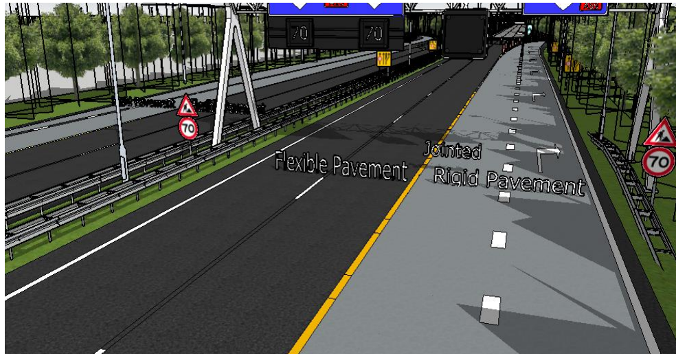
Figure 5.6. The idea of flexible and rigid pavement in the single road line.
