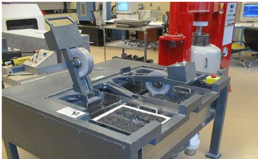
Figure 5.13. Hamburg wheel tracking device [70].
