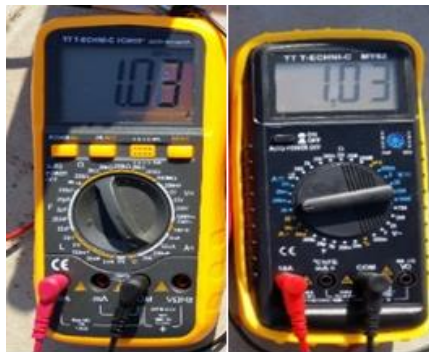
Figure 2.5. Two identical multimeters to measure current output.
