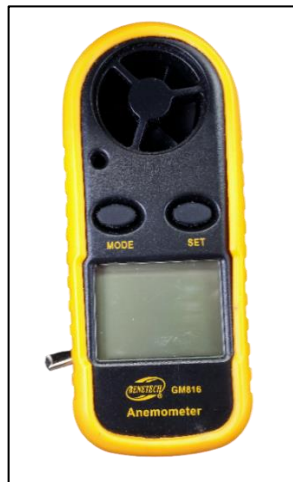
Figure 2.3. Anemometer Benetech GM816
