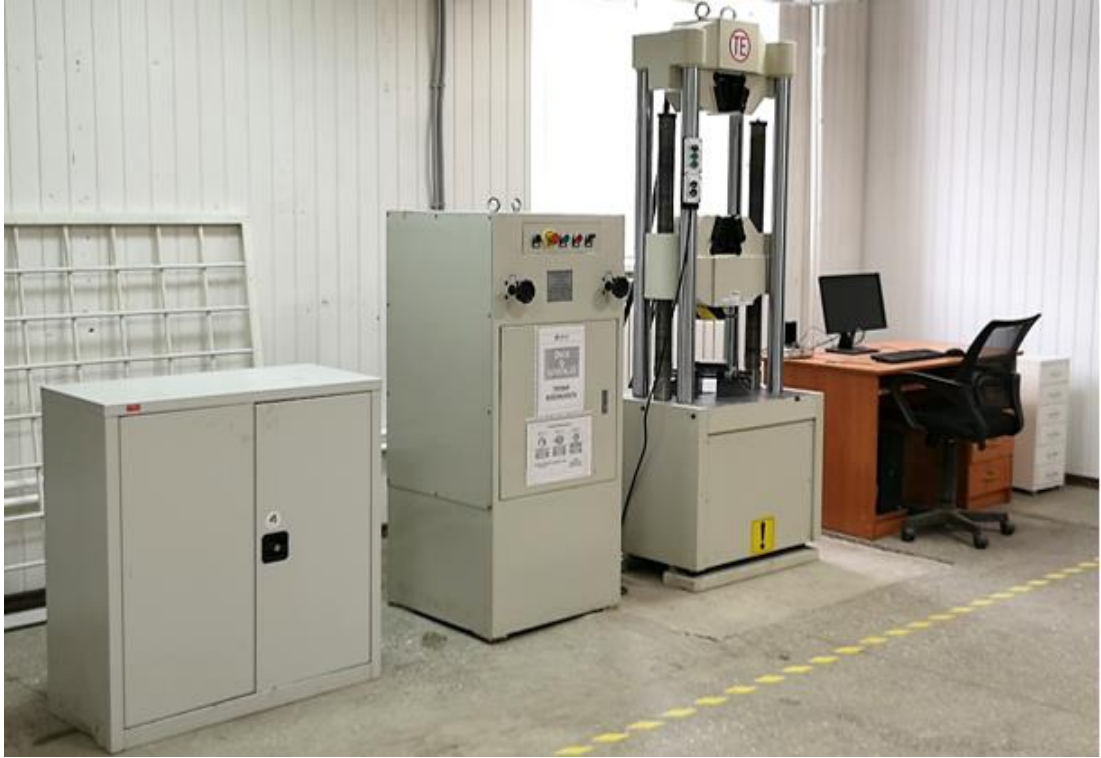
Şekil 5.13. Jinan Testing WAW-600B Universal tensile/bending hydraulic test machine”.
