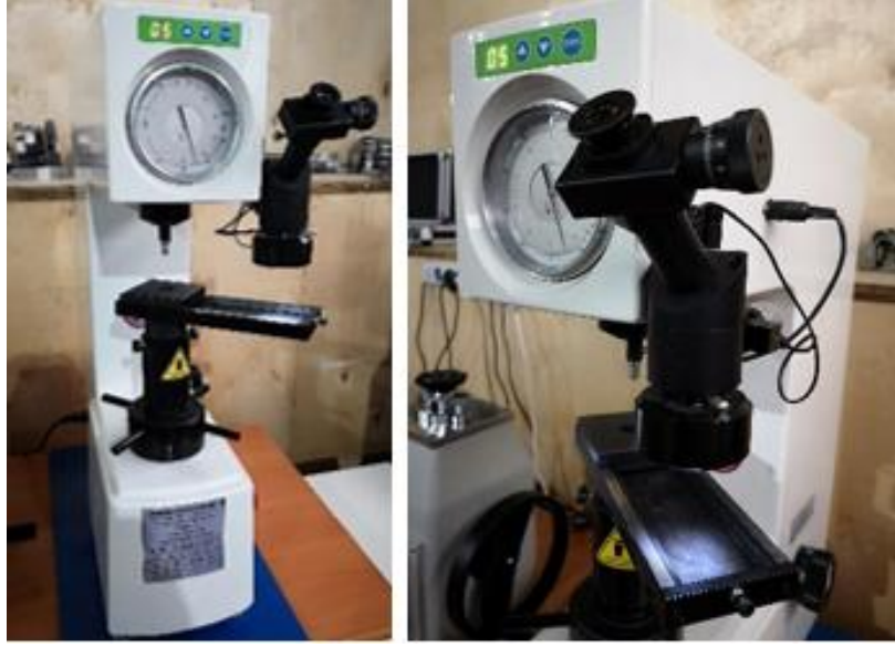
Şekil 5.12. Jinan Testing HBRV-187.5 Brinell rockwell vickers hardness tester.
