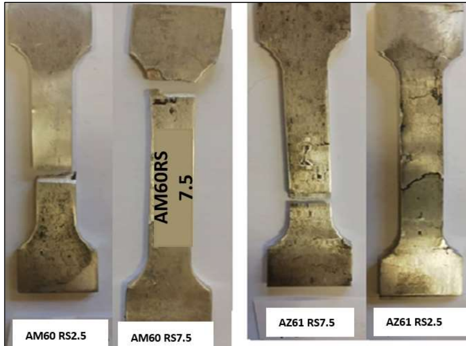
Figure 5.6. Tensile test specimens of hot rolled specimens.
