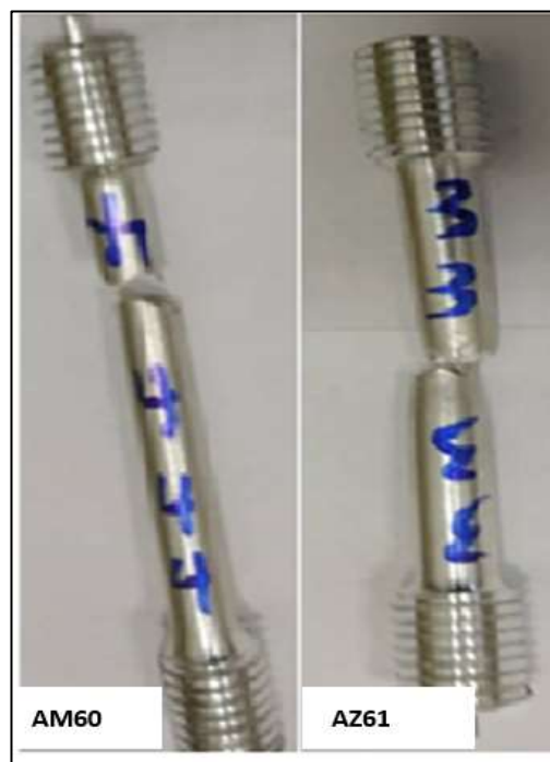
Figure 5.7. Extruded tensile test sample.
