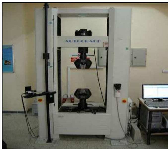
Figure 4.9. Shimadzu AG-IS 50 kN tensile tester for tensile testing.
