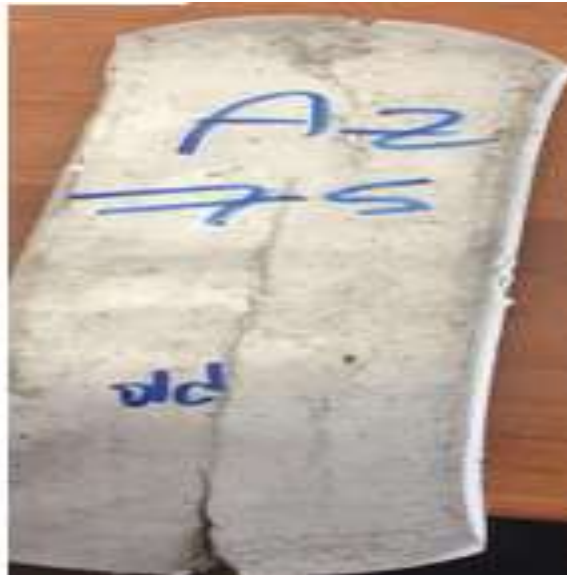
Figure 4.3. Rolling sample of magnesium alloys AZ61.
