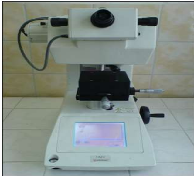
Figure 4.8. Shimadzu HMV2 microhardness tester for hardness measurements.
