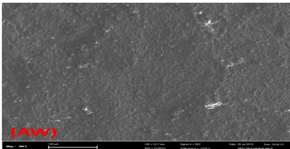
Figure 4.66. SEM images of wear marks: 800 °C, 8h - Ag@PVP.
